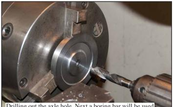
Drilling out the axle hole. Next a boring bar will be used to finish the bore
