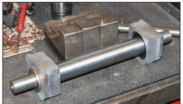
The ball bearings have been pressed on the axles, the boxes and thrust washers are in place, now where did I leave those wheels? (see page one for final assembly)
