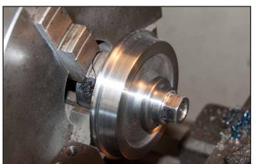
Wheel in process of flange machining, the tapered tread is finished. The wheel will be removed from the fixture and the other side of the flange will be formed.
