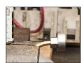
The originals right front, the new ones left front, other holders in the background. They hold the die with the cutting facing outwards and are guided by pins held in the tail-stock.
