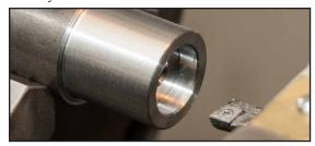
Took the part to the milling machine and drilled #35 and tapped it 6-32, and it is 0.125" form the outer edge, which should also
