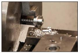
tail-stock to align the part square in the 3 jaw chuck. Basically the tail-stock was brought up to the part and the part held tight against the face of the chuck in the tail-stock and then the 3 jaw is tightened. This holds the part square enough for this operation.
