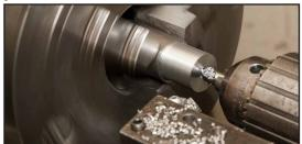
Bored a 0.814" dia hole 0.25" deep for the die and chamfered both edges. Hold the depth of the hole to within a thousandth or two. Both holes should be machined at the same time to ensure concentricity.
