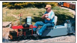
1.5" scale, 7.5" gauge Clishay locomotive and riding car. Engine is a two cylinder double acting 1 1/4x1 1/2". Boiler upgraded from the original 8" diameter water tube to a steel 10" diameter propane fired fire tube boiler with 73 1/2" copper fire tubes. Pneumatic FWD/REV shift and brakes on locomotive. Usual Accessories: working headlight, bell, new whistle, two new relief valves, engine driven feed pump and a hand pump. New body and trucks on riding car.
