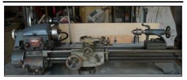
Wards (Logan) Power-Kraft Model 25TLC-2136 Back Geared Screw Cutting Lathe with Quick-change Gear Box 10" Swing - 1-1/2"-8 #3 MT Spindle Bore 50" Bed Length - 31" Between Centers Spindle Bore 25/32
