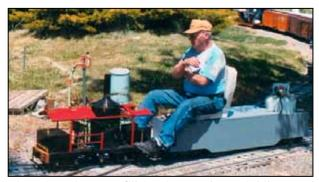
1.5" scale, 7.5" gauge Clishay locomotive and riding car. Engine is a two cylinder double acting 1 1/4x1 1/2". Boiler upgraded from the original 8" diameter water tube to a steel 10" diameter propane fired fire tube boiler with 73 1/2" copper fire tubes. Pneumatic FWD/REV shift and brakes on locomotive. Usual Accessories: working headlight, bell, new whistle, two new relief valves, engine driven feed pump and a hand pump. New body and trucks on riding car.
