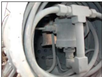
Inside smoke box includes tubing for drying the steam and heating the feed water. The copper colored flared piece at the rear is one of 2 that form the petticoat pipe and also act as resonance chambers to increase the sound of the engine.
