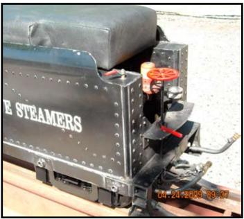
New Brakes on tender controlled by engine or hand wheel
