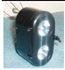
Dual Gyra-Light for sale. This light works on 3vdc and comes with wiring instructions and is ready to mount on your GP9 or SD9 in the vertical position or horizontal position on the later locomotives that used them. You only have to drill two #10 holes and another hole for the power cord. This dual gyralight comes with a 3 vdc power supply
